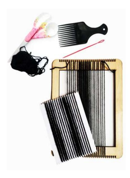
Looms and their tools are used to make woven fabric, and they come in all shapes and sizes. The core purpose of all looms is to keep the vertical warp strings taut for the weft yarn to be passed through from left to right and then beaten down to create the fabric. You will see different types of looms and tools in action in the video, however the ones that you will be using are listed below.
