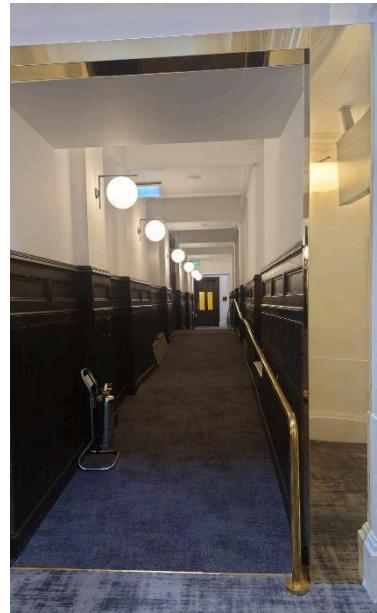
Once on the first floor, to cross over from one side of the building to the other you can use the ramp situated to the front of the building. The ramp is 152cm wide from the handrails to the opposite wall.
